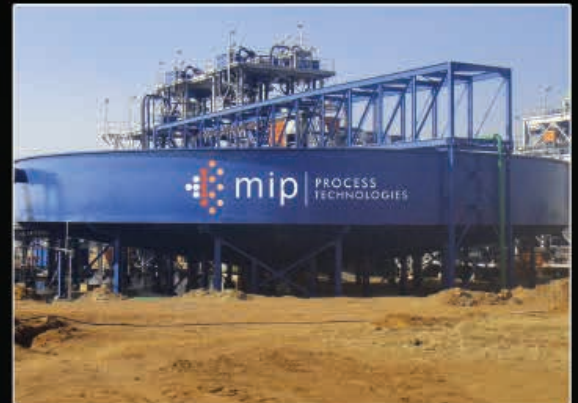
26m \phi Thickener in operation
